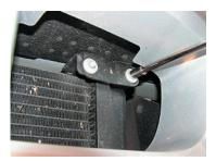
Move the assembly toward the radiator to unhook it from the back of the bumper and then gently lower it to gain access to the hoses.
