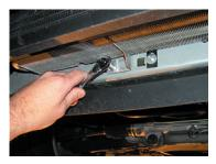
4. Remove the (4) bolts securing the factory heat exchanger to the front mounting brackets.
