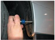
3. Remove the 2 bolts securing the power steering cooler and lower the cooler out of the way.
