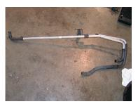
14. Remove the factory bracket assembly from the factory heat exchanger by removing the (4) bolts from the bottom bracket.
