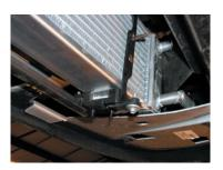
19. Position the molded hose so the 90 degree end attaches to the top fitting on the heat exchanger and the "elbow" end attaches to the coolant pump. Install and tighten the clamps.
