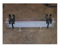
18. Install the AFCO Heat Exchanger assembly into the vehicle just like the factory unit was installed. Install the (4) bolts from the grill opening and tighten.
